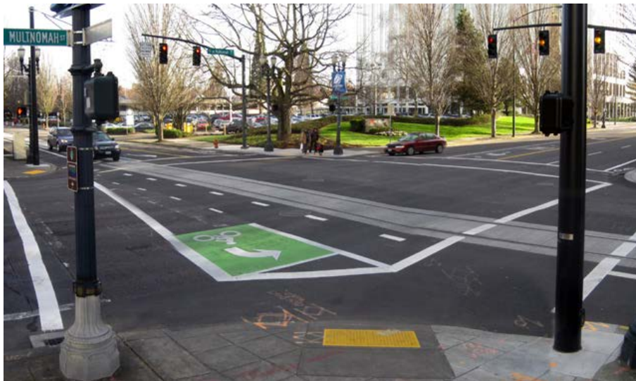
Figure 4-32: Example of two stage left turn box, Portland, OR Source: NACTO 2014 Urban Bikeway Design Guide
